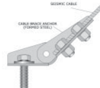
Figure 129: Cable attached with bolts to a bracket.
