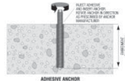
Figure 110: Adhesive anchor installation.
